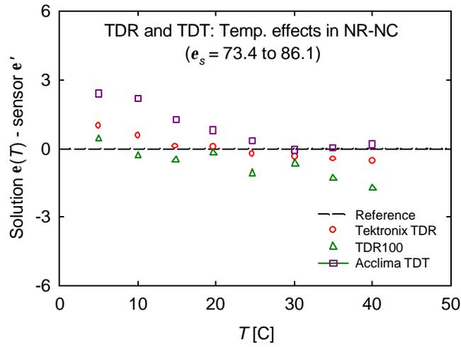
Figure 12: Deviation of higher frequency broadband sensing system  $\epsilon'$  predictions from modeled network analyzer  $\epsilon'$  measurements in NR-NC media with a temperature range of 5.05 to 40.0 °C (Table 2). The NR-NC sample used here has a  $\epsilon_s = 73.4$  to 86.1 (Table 2).
