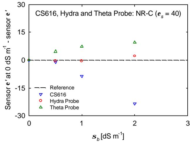
Figure 9: Deviation of lower frequency sensing system (excluding ECH<sub>2</sub>O Probe; see Figure 11)  $\mathbf{e}'$  predictions from the  $\mathbf{e}'$  prediction where electrical conductivity ( $\mathbf{s}_b$ ) = 0.0 dS m<sup>-1</sup> (reference) as NR-C sample  $\mathbf{s}_b$  increases from 0.0 to 2.0 dS m<sup>-1</sup>. The NR-C sample used here has a  $\epsilon_s = 40.0$  (Table 2).
