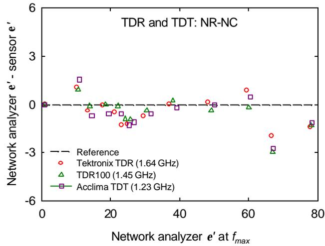
Figure 2: Deviation of higher frequency broadband sensing system  $\epsilon'$  predictions from the modeled network analyzer  $\epsilon'$  measurements (reference) in NR-NC media. The frequencies from which the reference  $\epsilon'$  measurements were taken are in parentheses and are maximum passable frequencies ( $f_{max}$ ).
