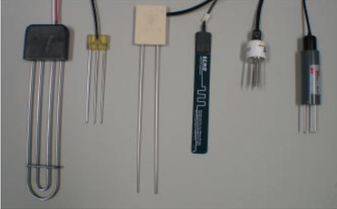
Figure 1: Probes of the sensing systems considered in the study are from left to right: Acclima Digital TDT Sensor, 3-rod TDR probe used with Tektronix TDR and TDR100 (0.15-m long 3.20 mm diameter rods, 12.0-mm rod spacing), CS616, ECH<sub>2</sub>O Probe, Hydra Probe and Theta Probe.
