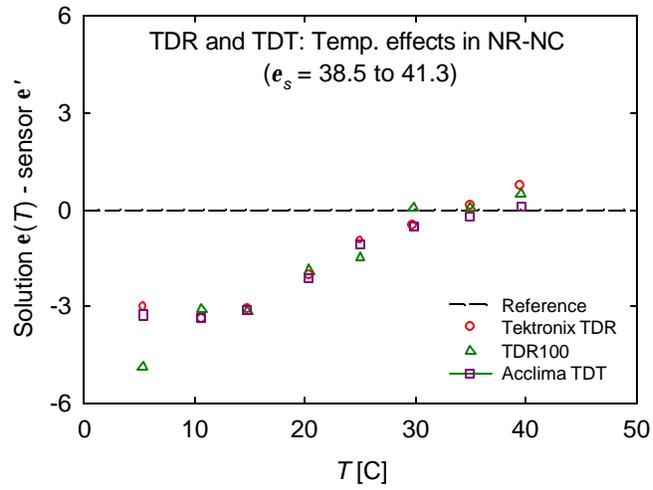
Figure 11: Deviation of higher frequency broadband sensing system  $\epsilon'$  predictions from modeled network analyzer  $\epsilon'$  measurements in NR-NC media with a temperature ( $T$ ) range of 5.38 to 39.5 °C (Table 2). The NR-NC sample used here has a  $\epsilon_s = 38.5$  to 41.3 (Table 2).
