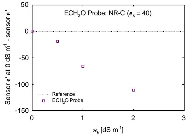
Figure 10: Deviation of ECH<sub>2</sub>O Probe  $e'$  predictions from the  $e'$  prediction where electrical conductivity ( $s_b$ ) = 0.0 dS m<sup>-1</sup> (reference) as NR-C sample  $s_b$  increases from 0.0 to 2.0 dS m<sup>-1</sup>.
