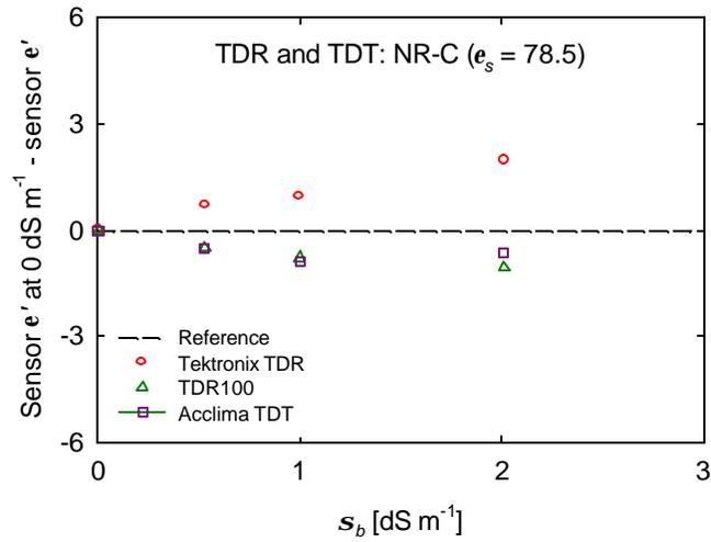
Figure 8: Deviation of higher frequency broadband sensing system  $\epsilon'$  predictions from the  $\epsilon'$  prediction where electrical conductivity ( $s_b$ ) = 0.0 dS m<sup>-1</sup> (reference) as NR-C sample  $s_b$  increases from 0.0 to 2.0 dS m<sup>-1</sup>. The NR-C sample used here has a  $\epsilon_s = 78.5$  (Table 2).
