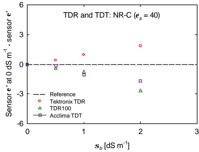
Figure 7: Deviation of higher frequency broadband sensing system  $\epsilon'$  predictions from the  $\epsilon'$  prediction where electrical conductivity ( $s_b$ ) = 0.0 dS m<sup>-1</sup> (reference) as NR-C sample  $s_b$  increases from 0.0 to 2.0 dS m<sup>-1</sup>. The NR-C sample used here has a  $\epsilon_s = 40.0$  (Table 2).
