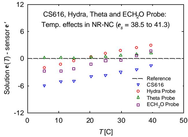
Figure 13: Deviation of lower frequency sensing system  $\mathbf{e}'$  predictions from modeled network analyzer  $\mathbf{e}'$  measurements in NR-NC media with a temperature ( $T$ ) range of 5.38 to 39.5 °C (Table 2). The NR-NC sample used here has a  $\epsilon_s = 38.5$  to 41.3 (Table 2).
